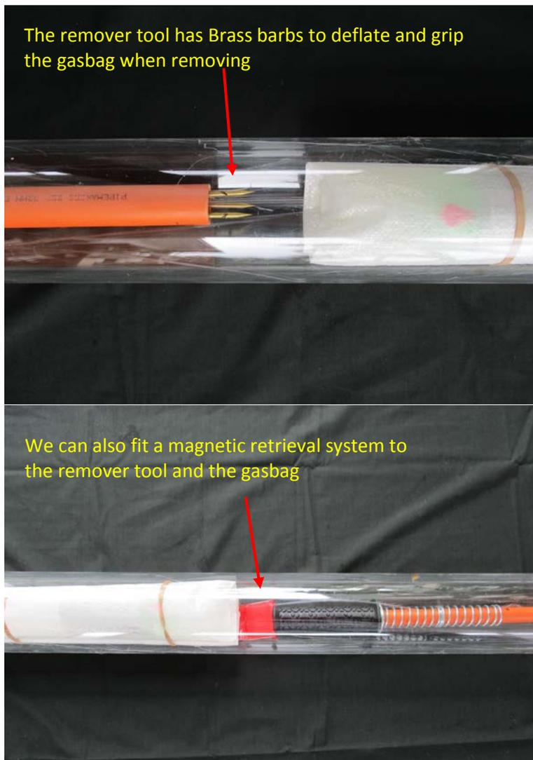
The remover tool has Brass bars to deflate and grip the gasbag when removing
